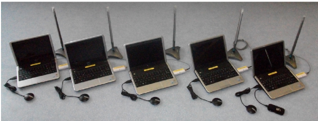
Figure 16: Experimental platform composed of mini Dell under Linux, external WiFi cards, external antennas and GPS.
