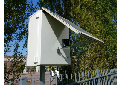
(c) RSU enclosed with energy harvesting unit and Xbee sensor
