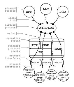
Figure 1: A node in the airplug architecture.
