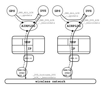
Figure 5: Messages exchanged for the discovering service DVS.
