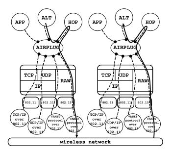
Figure 2: Integration of a new protocol in the airplug architecture. Here the HOP protocol is used by the ALT application.
